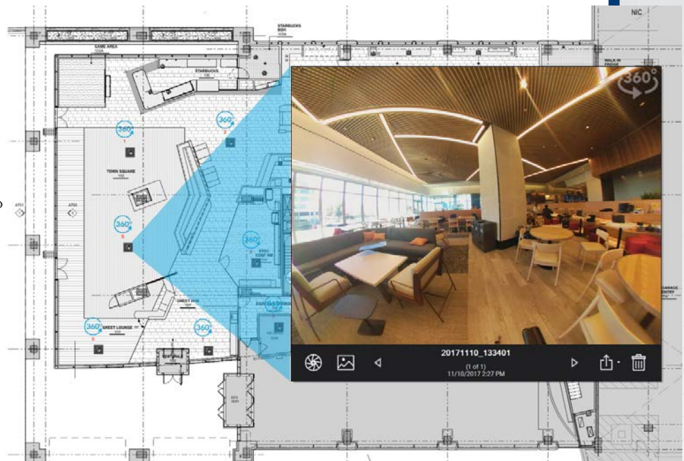
Figure 2: 360 image embedded in Bluebeam Revu PDF plan.
