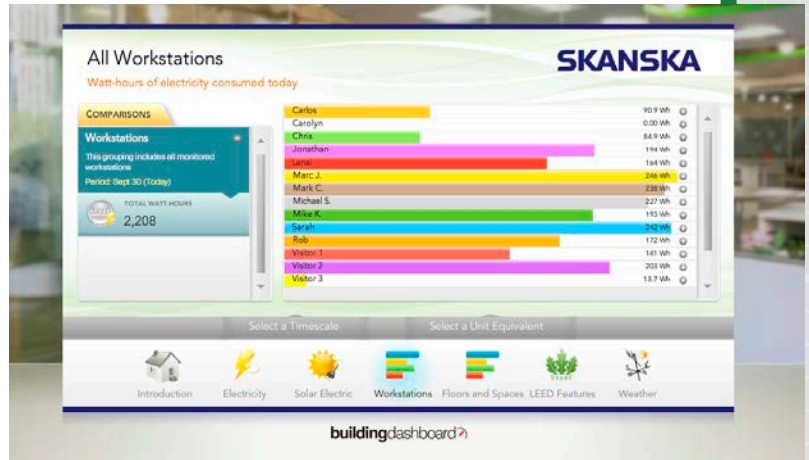
Enmetric plug-load monitoring system.
