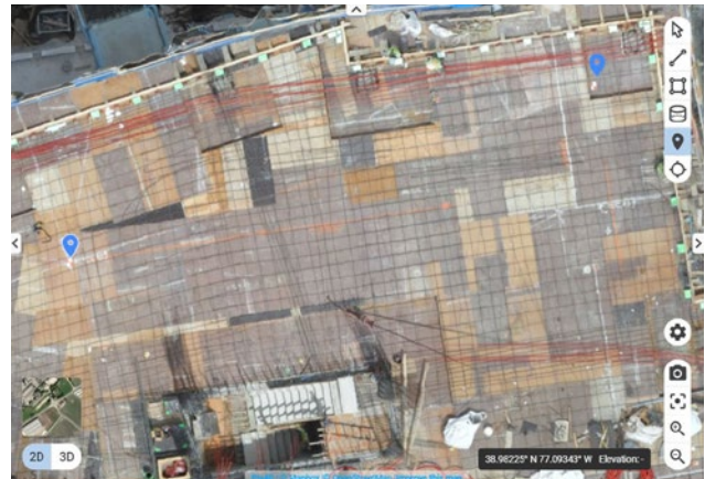
Figure 3: Physical targets are captured on the daily orthomosaic image and are marked on the online Pix4D account, Miller & Long Co.
